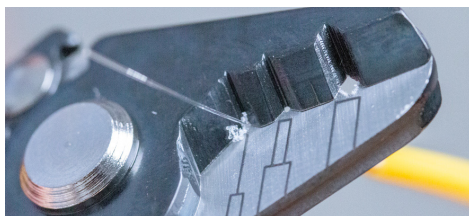
8 - Cleave Fiber with FC-600
